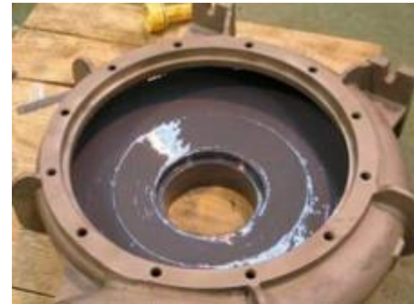
Pump after applying ARC coating system
