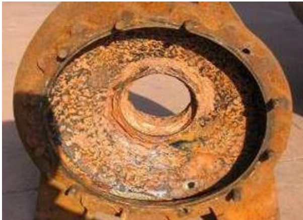
Pump before applying ARC coating system
